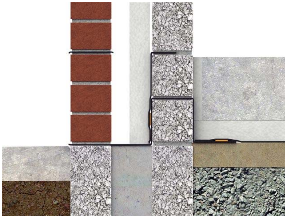
Figure 10: Detail showing floating slab
