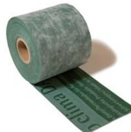
DA-S is a vapour check and airtight sealing strip manufactured from PP with a robust Polypropylene Protection Fleece. DA-S strips are glued to building substrates to maintain airtightness continuity at critical junctions. Rolls are 210mm wide and 100m long.
