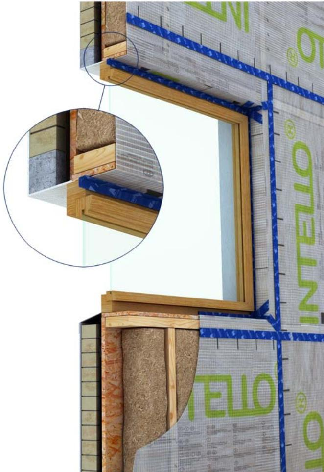
**Figure 2: Window Detail sealed with TESCON PROFIL**
