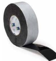
TESCON NAIDEC is a double-sided nail-sealing tape for use on the underside of a lath on inclined roofs to form a durable seal around nail or screw holes. Rolls are 50mm wide and 20m long.
