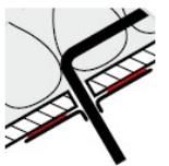
Conduit grummets are to be used for conduits or thick cables (diameter 15 to 30mm).
