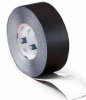
TESCON INVIS is designed to conceal sealed overlaps in SOLITEX WA when one is planning a cladding with opened joints. It is a multipurpose tape to seal overlaps between foil and fleece membranes and joins between such membranes and smooth, non-mineral surfaces. It is also suitable for sealing butt joints between wood based panels such as OSB. Rolls are 60mm wide and 30m long.
