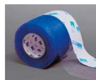
CONTEGA PV forms a high quality bond between vapour check, wood based panels (e.g. OSB) and masonry. The airtight bond is completed once the light blue PET fleece is plastered into place. The latex-reinforced layer increases the strength of the adjoining plasterwork.
