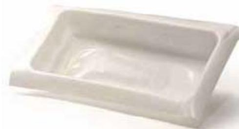
INSTAABOX is an installation box for creating space for junction boxes etc. in buildings without a service void behind the dry-lining. It is designed for making airtight connections on vapour check and airtightness layers, and can be used on all common substrates in construction.
